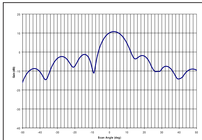
Elevation Radiation Pattern (Model AA90)
